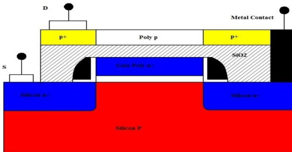
Fig.1 Structure of a Bulk Double Gate Field Effect Transistor
