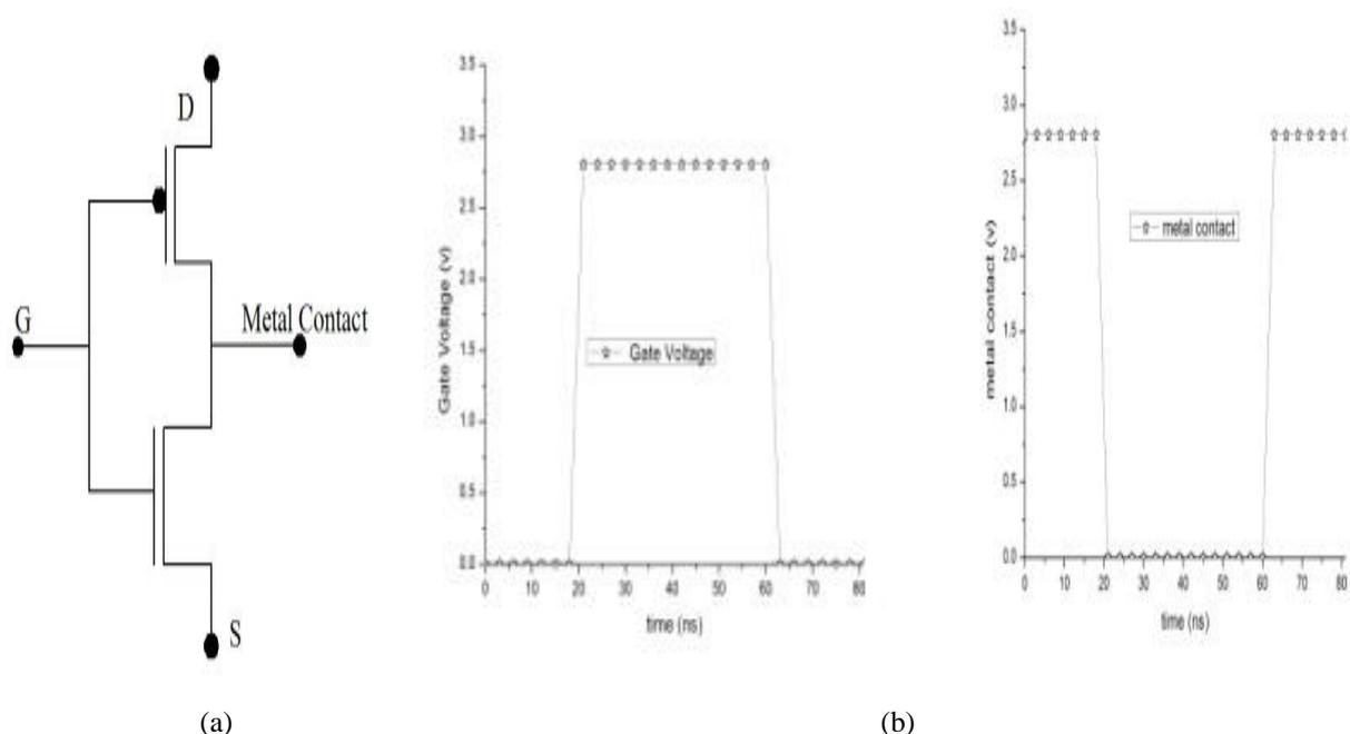
**Fig.2 nMos Double gate equivalent circuit (a), and TCAD device simulation results (b) obtained by applying a rectangular voltage pulse to the gate of a Double Gate device drain at  $2.8\text{V}$  and source connected to ground. The solid line shows the behavior of the metal contact terminal.**
