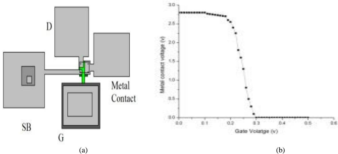
**Fig. 3. Micrograph of 1.5μm Double Gate MOS device (a) and DC measurements of the metal contact terminal voltage as a function of the gate voltage in inverter mode (b), i.e. with the SB(Source Body) terminal connected to ground and drain at 2.8V**
